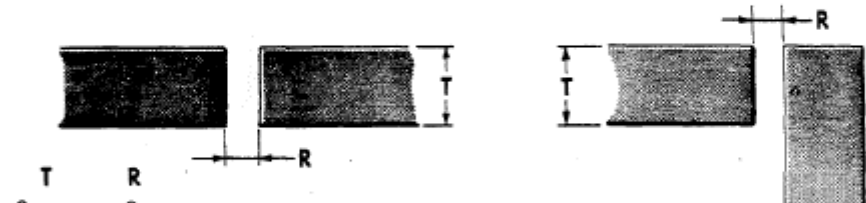
Square groove welded on both sides
